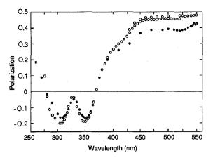
Fig. 1. Excitation polarization spectra of eosin-5-maleimide adducts of N-acetylcysteine in glycerol (open symbols) and myosin in buffer (closed symbols). Both samples were thermostatted at 5°C, Excitation bandwidth was 2 nm and emission was monitored through a cutoff filter (Schott GG089) which passed wavelengths longer than 550 nm.
